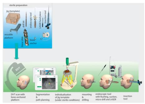
Figure 24: Robofig. Workflow of the robotic minimally invasive cochlear implantation
