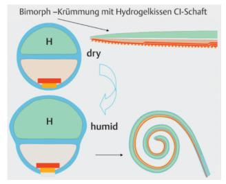
Figure 42: Hydrogel-based self-bending electrode (according to Doll and Stieghorst 2015)
