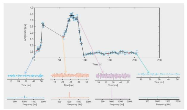
Figure 21: Intraoperative cochlear monitoring. Registration of Cochlear Microphonics. Amplitude decline during insertion of the electrode in a case of cochlear damage.
