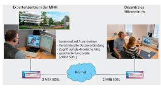
Figure 6: Technical realization of remote fitting (according to A. Büchner). Expert center of the Hannover Medical School. Decentral hearing center, based on the Auric system, coded data connection, secured bandwidth (2 Mbit SDSL)
